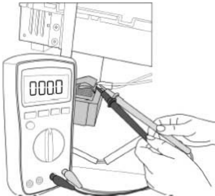
Fig. 43 —Test Resistance of Reactor with Multimeter
